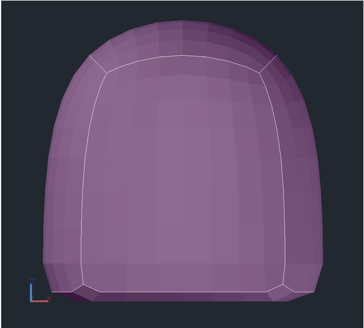
The cube with subdivision level of 3 and crease values of 1.0:
