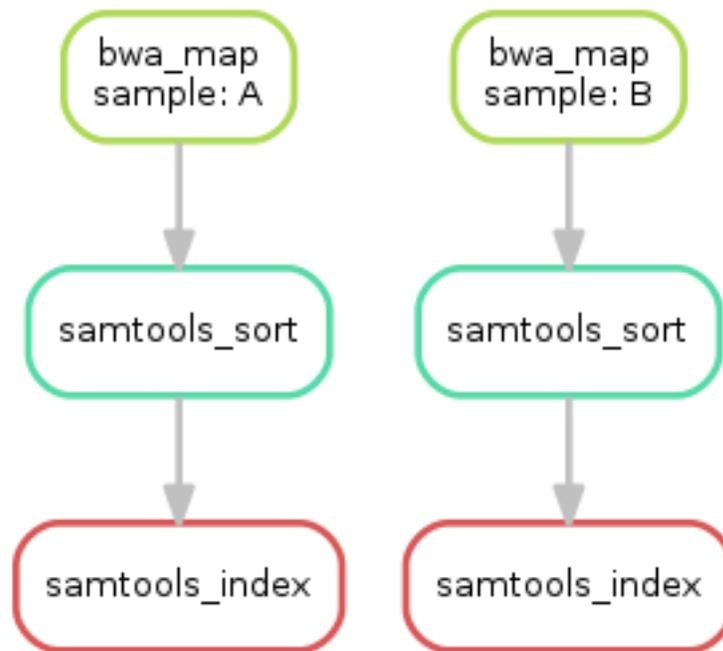
The DAG contains a node for each job with the edges connecting them representing the dependencies. The frames of jobs that don't need to be run (because their output is up-to-date) are dashed. For rules with wildcards, the value of the wildcard for the particular job is displayed in the job node.
