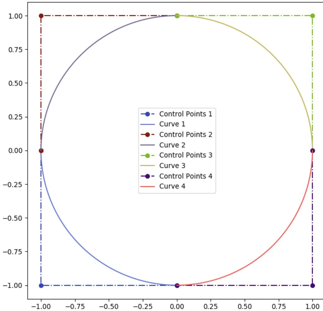
The following is a circular curve generated with 7 control points as illustrated on page 301 of *The NURBS Book* (2nd Edition) by Piegl and Tiller. There is also an option to generate this shape via `geomdl.shapes` module.
