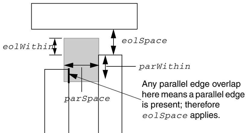
b) EOL space rule with PARALLELEDGE is triggered only if there is a parallel edge that overlaps inside the illustrated shaded box.
