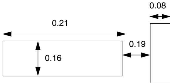
e) Violation, it can happen in EOL when the conditions are fulfilled. With span length of 0.21, 0.2 spacing is needed
