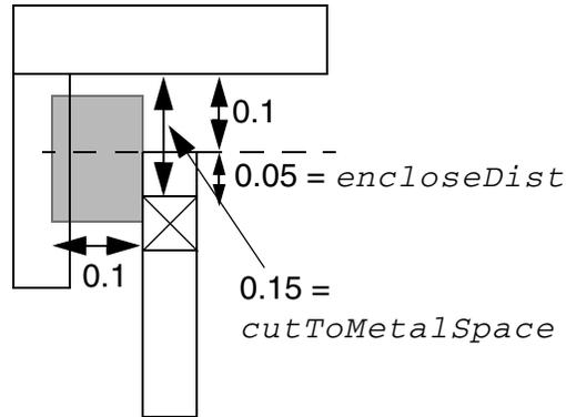
b) Violation. Meets min length, has parallel edge, cut enclosure  $encloseDist < 0.06$ ,  $cutToMetalSpace < 0.16$ , so needs 0.15  $eolSpace$ .
