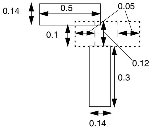
e) OK, it fulfills the end-to-line EOL spacing of 0.1, and the 2 EOL edges do not have common parallel run length such that end-to-end EOL spacing is ignored.
