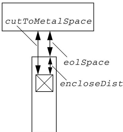
c) EOL with ENCLOSECUT rule is triggered if EOL edge has a cut edge that has  $< encloseDist$  enclosure, and the cut edge is  $< cutToMetalSpace$
