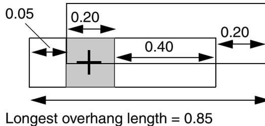
f) Okay. Overhang length  $\geq 0.70$ . (The center of the via cut is where the total overhang length is measured.)
