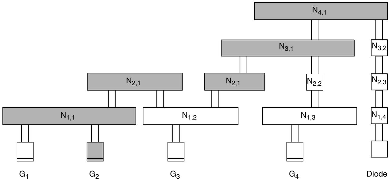
The path of the current between gate  $G_2$  and node  $N_{4,1}$  is shaded.
