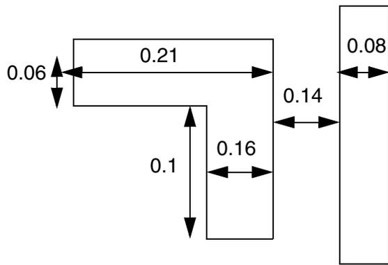
a) Violation, the continuous parallel run length of  $0.1 + 0.06 = 0.16 (> 0.15)$ , and top & bottom edges on the left have span length  $> 0.1$ , 0.15 spacing is needed
