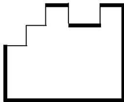
The `EXCEPTSAMECORNERS` definition of same-corners edges refers to any edge that ends in two convex or two concave 90-degree corners. All of the thick edges in the object above have same-corner edges, and would not be checked by this rule.. "Stair-step" edges are shown in thin lines.
