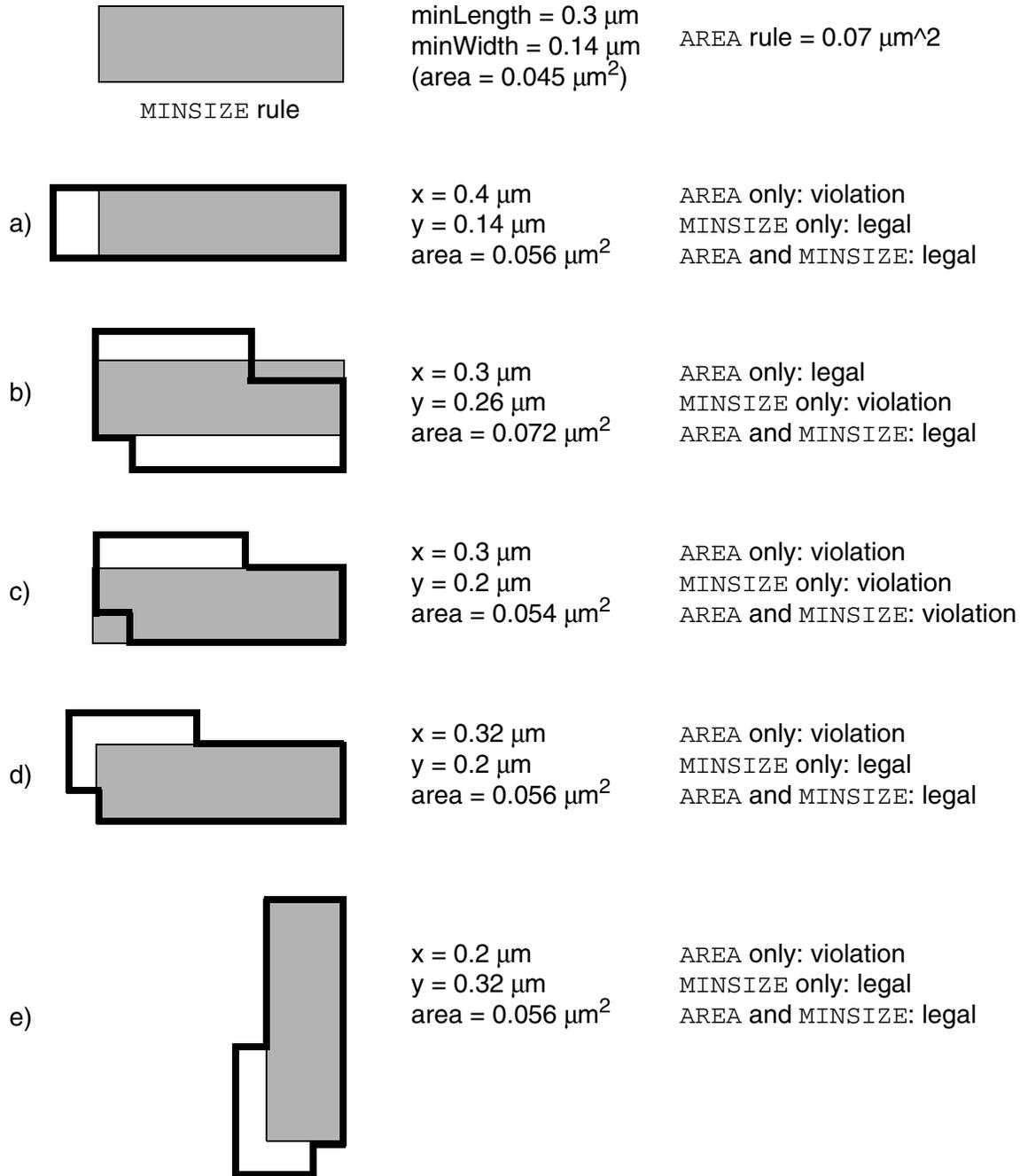
The following statement defines a `MINSIZE` rule that specifies that every polygon must have a minimum area of 0.07  $\mu\text{m}^2$ , or that a rectangle of 0.14 x 0.30  $\mu\text{m}$  must be able to fit within the polygon, or that a rectangle of 0.16 x 0.26  $\mu\text{m}$  must be able to fit within the polygon:
