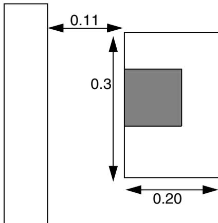
a) Okay. Width  $\geq 0.2$ , but spacing to neighbor is  $\geq 0.11$ , so edge enclosure rule is not required. Cut meets the normal 0.00 0.05 enclosure rule.
