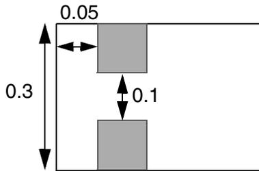
a) OK. Extra-cut is  $\leq 0.2$  away, with PRL  $> 0$ , so use min-width rule, both cuts meet the 0.05 enclosure rule of 0.05
