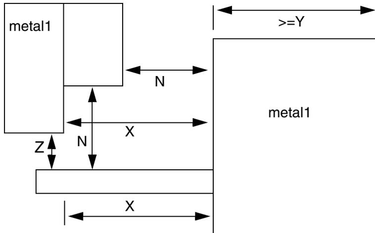
In the following example, the 0.5  $\mu\text{m}$  spacing applies for the first 1.0  $\mu\text{m}$  of the stub sticking out from the large object. This rule only applies to the stub wire; the previous rule must be included for the wide wire spacing. The `SPACING 0.5 RANGE 2.01 2000.0` statement is required to get extra spacing for the wide-wire itself.
