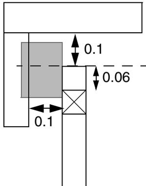
c) No violation. Meets min length, has parallel edge, but cut enclosure  $encloseDist \geq 0.06$ , so do not check  $eolSpace$ .
