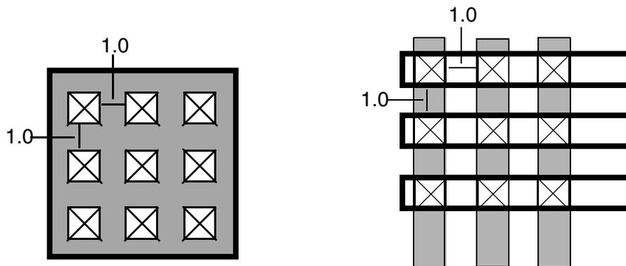
a) Allowed if cuts are on power or ground nets. Violation if cuts are on signal net.
