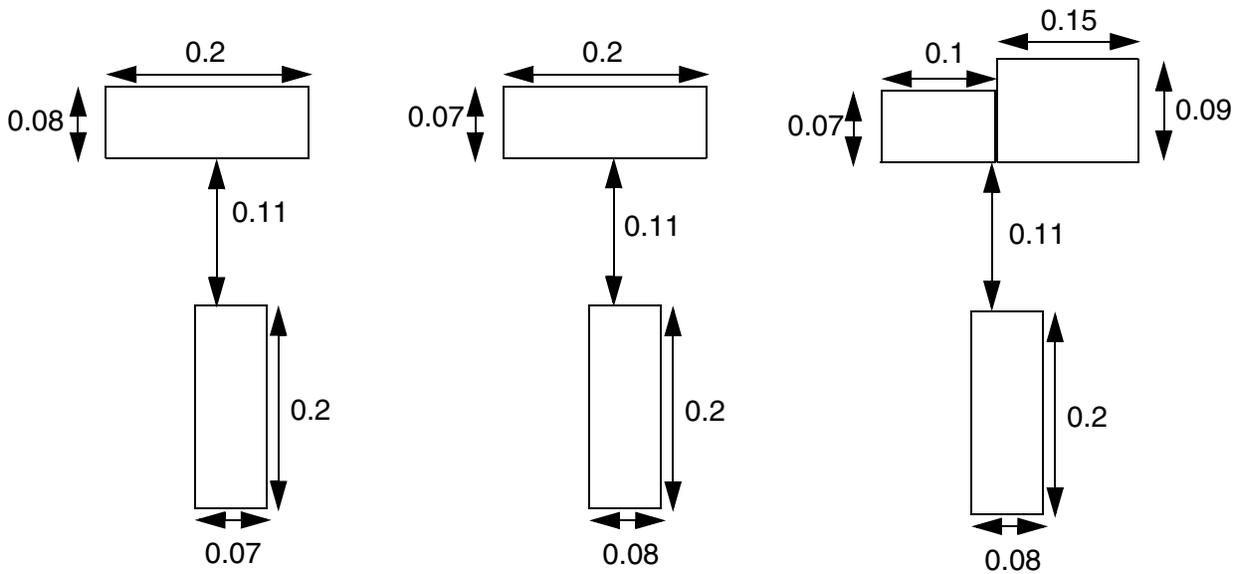
c) OK, opposite wire width  $\geq 0.08$ , and the rule does not apply
