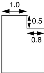
a) Violation, an edge <  $0.6\ \mu\text{m}$  long has adjacent edges <  $1.0\ \mu\text{m}$ .
