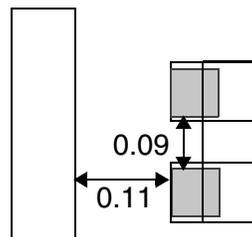
f) Violation, the common metal shapes covering the entire length of the projection between the cuts
