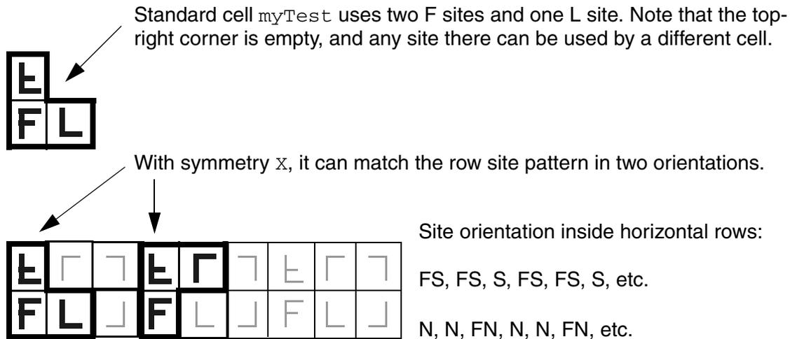
The following statement includes the gate-array site pattern syntax. It uses two F sites in a row with N (North) orientation.
