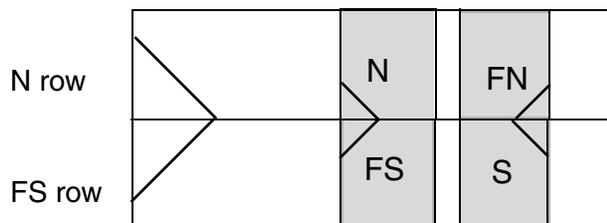
The following examples describe typical combinations of orientations for standard cells. Applications typically create only N (or FS for flipped) row orientations for horizontal standard cell rows; therefore, the examples describe these two rows.
