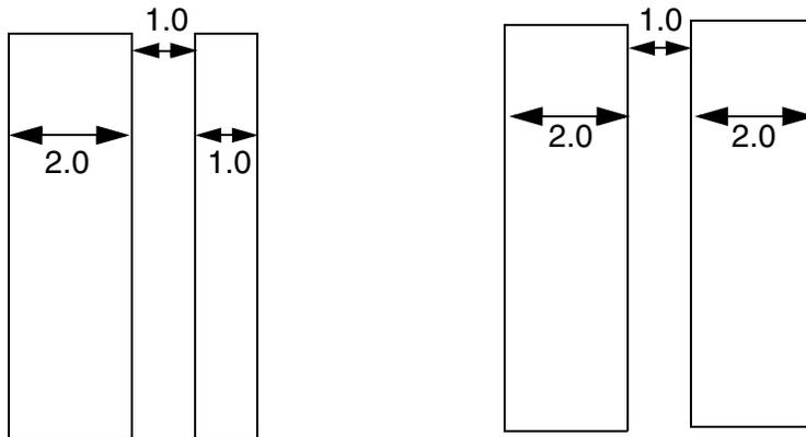
a) Okay if both wires are the same net and are either a power or ground net.
