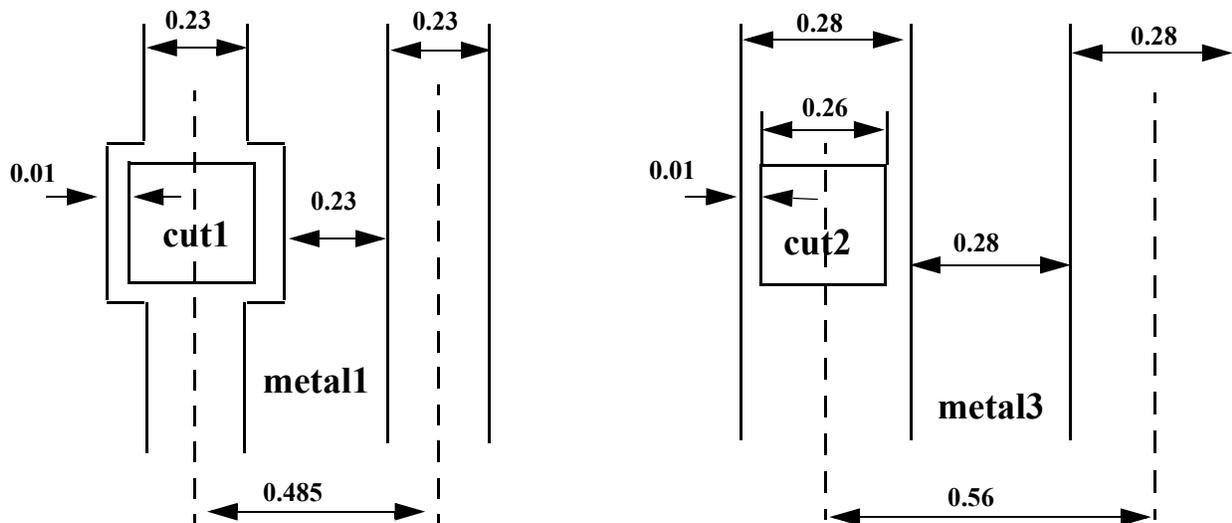
Although the minimum `metal1` routing pitch is 0.485 $\mu$ m from the design rule, you should use 0.56 $\mu$ m instead, to match the `metal3` routing pitch in the same preferred direction.
