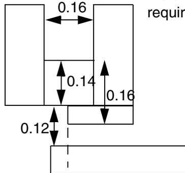
e) Violation. Notch metal width is  $< 0.15$  for part of the overlap; therefore 0.14 spacing is required.
