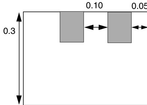
d) Okay; extra cut is  $\leq 0.2$  away; therefore, use min-width rule, and both cuts meet min-width enclosure rule of 0.0 and 0.5.
