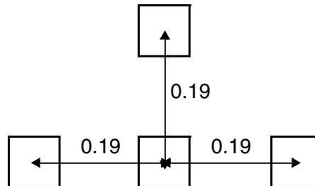
d) Violation. Three perfectly aligned neighbor cuts would trigger the rule spacing of 0.2
