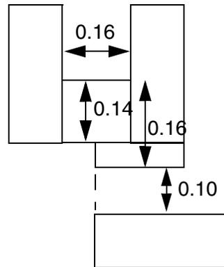
d) Okay. Notch metal width is  $\geq 0.15$  for the overlap; therefore extra space is not required.
