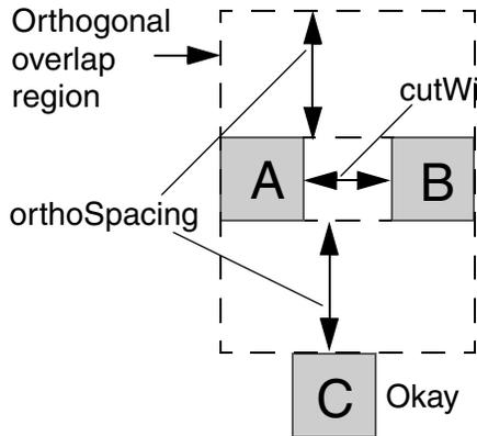
a) If two cuts < cutWithin apart and overlap, then no other cut is allowed inside the orthogonal overlap region.
