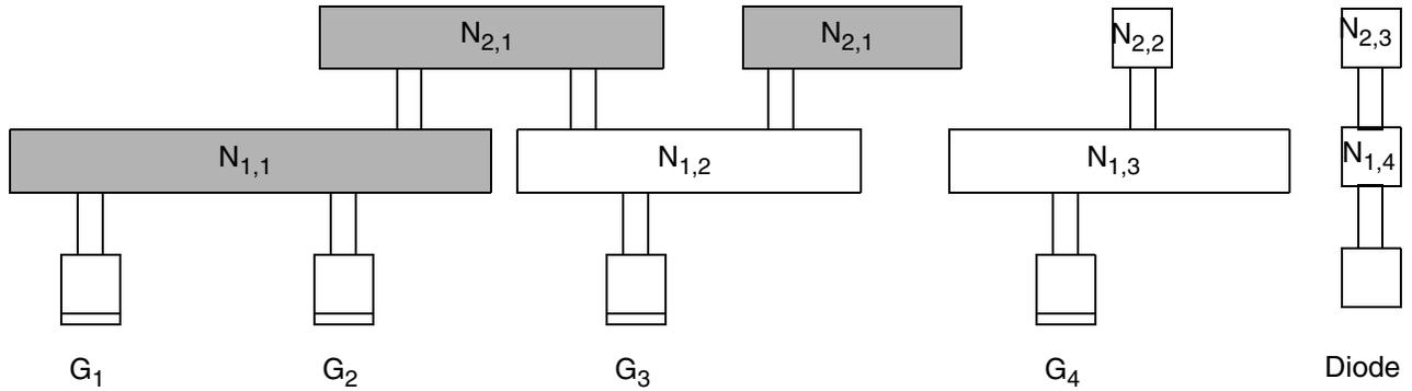
The path of the current between gate  $G_1$  and node  $N_{2,1}$  is shaded.
