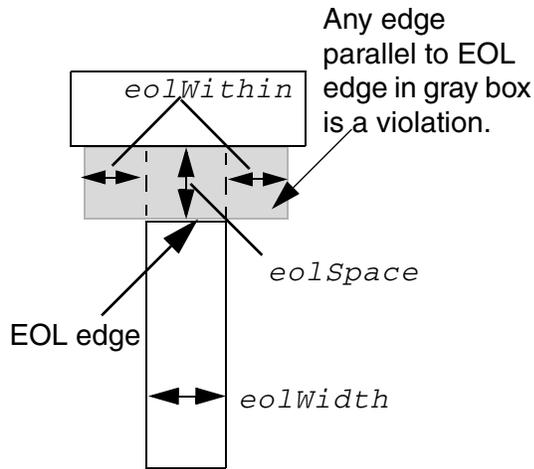
a) Basic EOL rule: EOL width  $< eolWidth$  requires  $\geq eolSpace$  beyond EOL edge to opposite edges to either side by  $< eolWithin$  distance (gray box).
