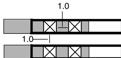
c) Allowed if cuts are on the same power or ground nets. Violation if cuts are on signal nets, or different nets.
