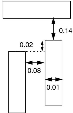
b) OK, the combined EOL wire width & the gap of the parallel edge is 0.17 ( $\geq 0.16$ ), and the EOL rule does not apply
