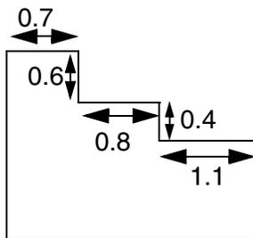
a) Violation, the convex corner of 0.4 and 0.8 edges is between 2 concave corners, and their lengths are smaller than 0.6 and 1.0 correspondingly
