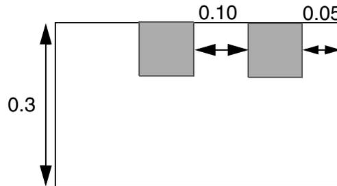
d) Okay. Extra cut is close enough so just need 0.0 0.5 enclosure. Violation if NOSHAREDEDGE is specified; extra cut has shared edge, so wide-wire enclosure of 0.03 0.03 is required.
