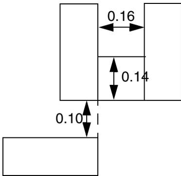
c) Okay. No overlap with notch above; therefore only default spacing of 0.10 required.
