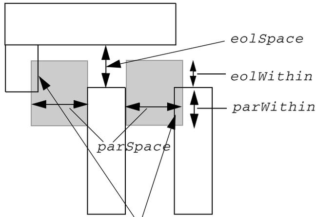
There must be parallel edges in both areas to trigger two-edge rule.
