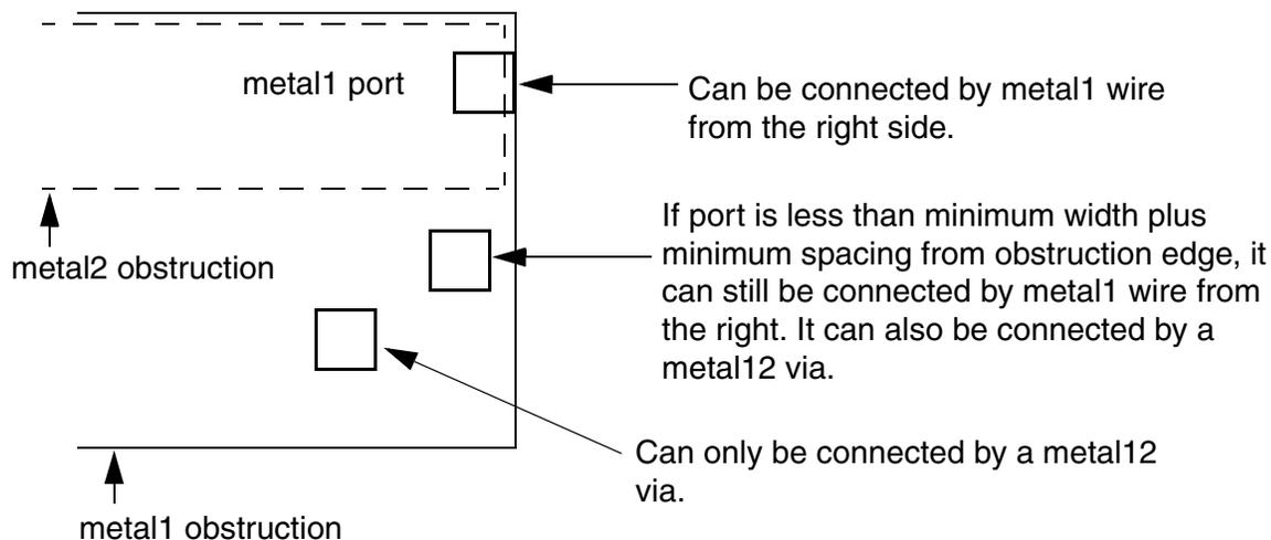
If a port is on the edge of the obstruction, a wire can be routed to the port without violations. Pins that are partially covered with obstructions or in apparent violation with nearby
