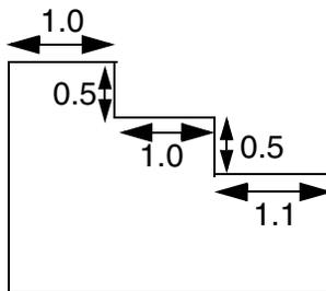
b) Okay, all edges <  $0.6\ \mu\text{m}$  long have  $\geq 1.0\ \mu\text{m}$  adjacent edges.
