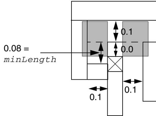
f) Violation. The  $minLength = 0.08$  means no left parallel edge, but the right side has a parallel edge, so needs  $0.15$  *eolSpace* or  $cutToMetalSpace \geq 0.16$ .
