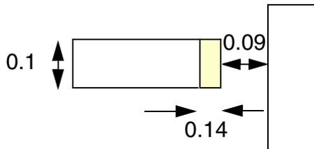
a) Violation, 0.14 extension is applied for width < 0.11, and 0.1 spacing is required after the extension
