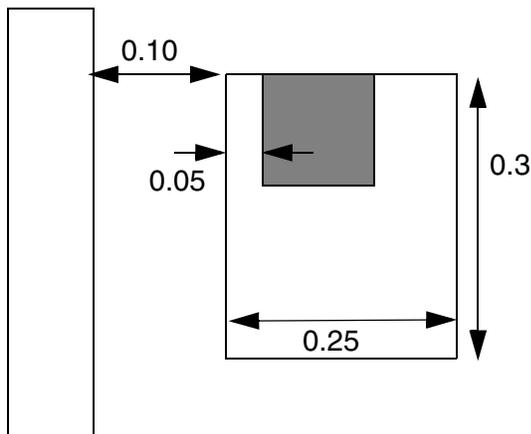
c) Okay. Width  $\geq 0.2$ , spacing to neighbor is  $< 0.11$ , parallel length is  $> 0.25$ , so edge enclosure rule of 0.02 is required and met. Cut also meets the normal 0.00 0.05 enclosure rule.
