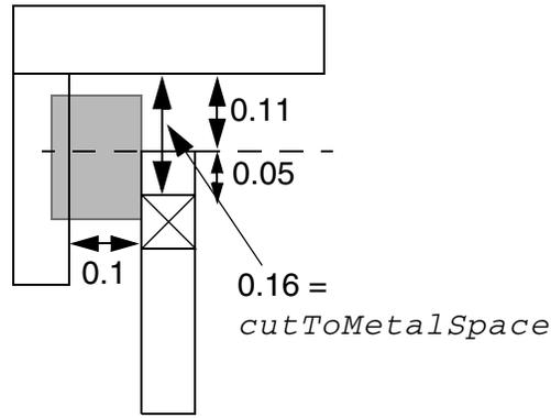
d) No violation. Meets min length, has parallel edge, cut enclosure  $encloseDist < 0.06$ , but  $cutToMetalSpace \geq 0.16$ , so do not check  $eolSpace$ .
