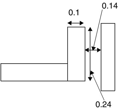
a) No violation. The 0.24 edge is not a valid EOL edge with the `EQUALRECTWIDTH` keyword since its length is not the same as the wire width of 0.1.
