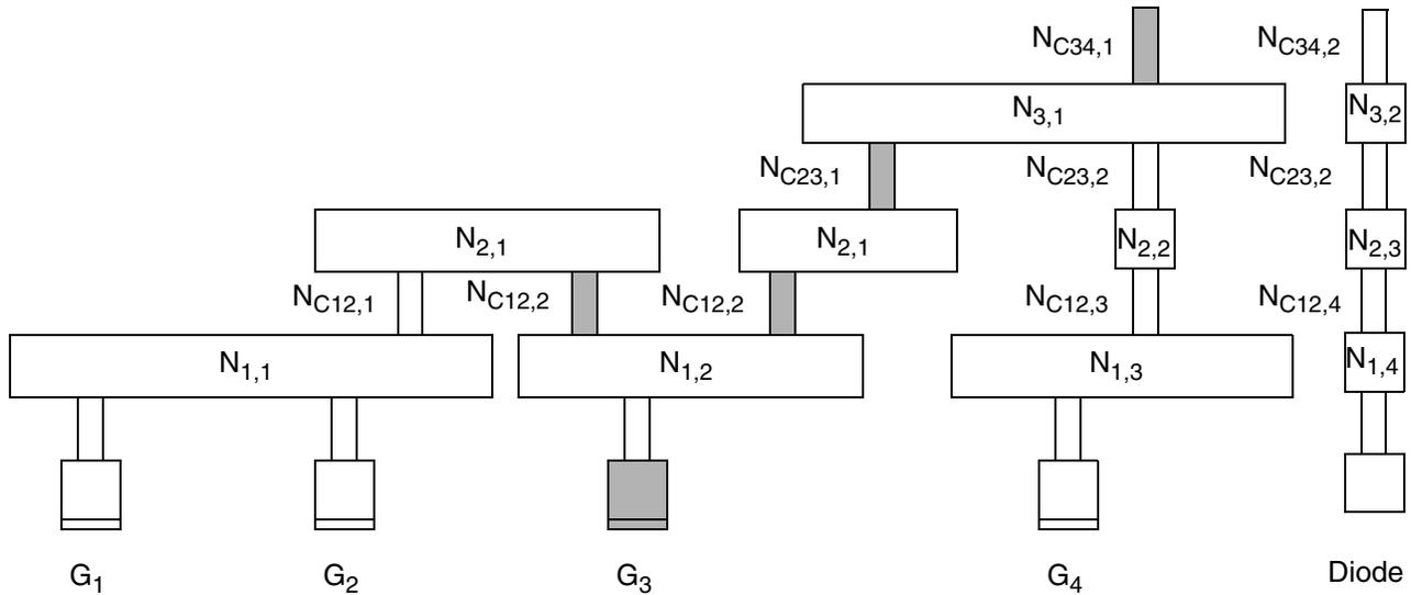
The router calculates the CAR with respect to gate  $G_3$  after the cut  $C_{34}$  process step as follows:
