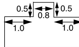
c) Violation, the edges <  $0.5\ \mu\text{m}$  have an adjacent edge <  $1.0\ \mu\text{m}$ .
