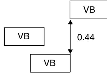
b) OK, the right VB does not have side by side parallel edge overlap > 0
