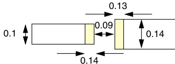
b) Violation, for end-to-end situation, 0.14 extension is applied for width < 0.11 on the left, 0.13 extension is applied for width  $\geq$  0.11, and 0.1 spacing is required
