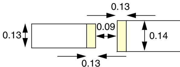
c) Violation, for end-to-end situation, 0.13 extension is applied for both wires with width  $\geq$  0.11, and 0.1 spacing is required
