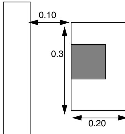
b) Violation. Width  $\geq 0.2$ , spacing to neighbor is  $< 0.11$ , parallel length is  $> 0.25$ , so edge enclosure rule of 0.02 is required but not met.
