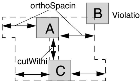
d) The rule applies in both the X and Y directions. In this case, the horizontal overlap of A and C makes B a violation.
