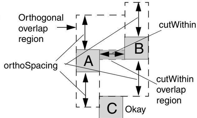
b) Orthogonal overlap region is computed from the cutWithin overlap region and cuts extended out orthogonally by orthoSpacing.
