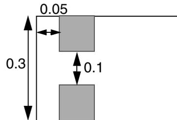
f) Okay. Okay for NOSHAREDEDGE also. Extra cut is  $\leq 0.2$  away, there is no shared edge; so use minimum width rule; both cuts meet the minimum width enclosure rule of 0.0 0.05.
