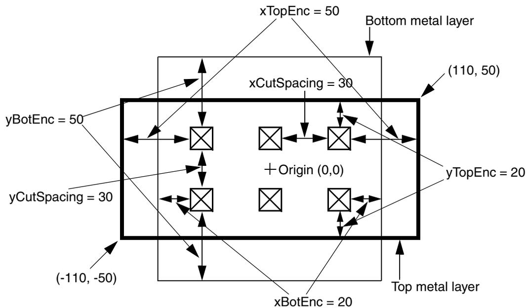
The same via rule with the following `ORIGIN` parameter shifts all of the metal and cut rectangles by 10 in the x direction, and by -10 in the y direction (see [Figure 4-17](#) on page 330):
