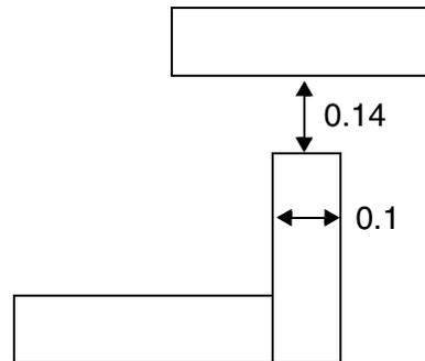
b) Violation. The 0.1 edge is a valid EOL edge, even with the `EQUALRECTWIDTH` keyword, and EOL spacing is  $< 0.15$ .
