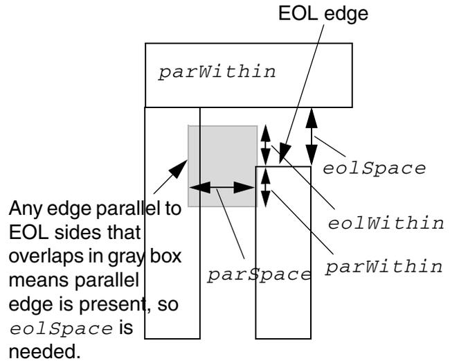
b) EOL with PARALLELEDGE is triggered only if an EOL side also has a parallel edge  $< parSpace$  and  $< eolWithin$  above, or  $< parWithin$  below, EOL edge (gray box). If  $minLength$  is given, and the EOL side is  $< minLength$ , the parallel edge does not matter, and no extra space is needed.
