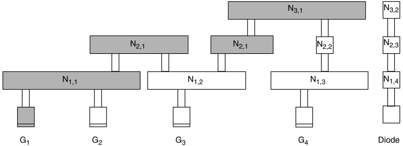
The path of the current between gate  $G_1$  and node  $N_{3,1}$  is shaded.
