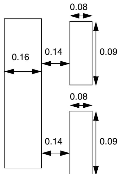
d) OK, parallel run length is not continuous, and each of the individual ones of  $0.09 \leq 0.15$  would not trigger the rule
