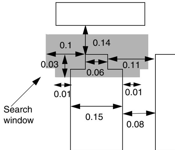
d) Okay, the parallel edge is searched by extending the outline of the wire dynamically based on the wire width. Hence, 0.1 ( $0.16 - 0.06$ ) on top, and 0.01 ( $0.16 - 0.15$ ) on bottom.
