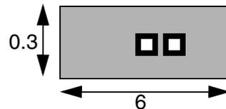
d) Okay; `MINIMUMCUT 2` `WIDTH 0.24` rule applies. The `WITHIN` rules do not apply when direct via is dropped.
