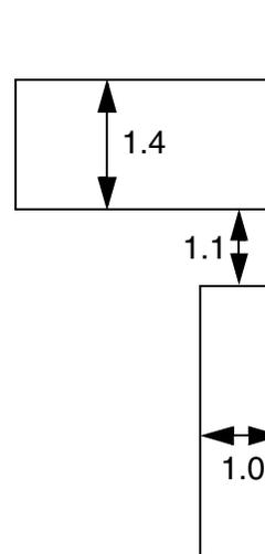
d) No violation. Perpendicular edge is not "seen" by EOL edge, so it is not checked.
