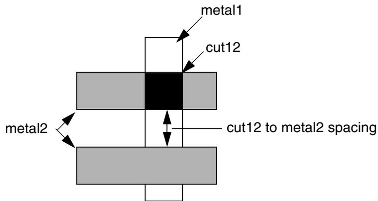
The "SPACING 0.15 LAYER metal2 ;" rule only applies to outside edges; therefore, no violations between cut12 and the top metal2 shape will occur. Only the spacing to the bottom metal2 shape is checked.
