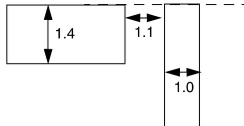
b) No violation. Perpendicular edge is not "seen" by EOL edge, so it is not checked.
