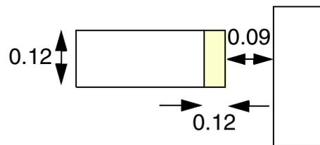
d) Violation, 0.12 extension is applied for width  $\geq$  0.11 for end-to-side, and 0.1 spacing is required
