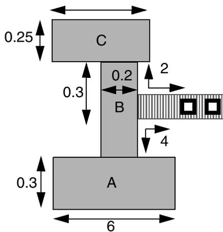
c) Okay; the area of C only needs 2 cuts, and the area of A needs 3 cuts, but the cut is farther than the `WITHIN` distance of 3, and it also fulfills the 2 cuts requirement. Same situation occurs if a 2 cut via is directly connected to B instead of a wire.
