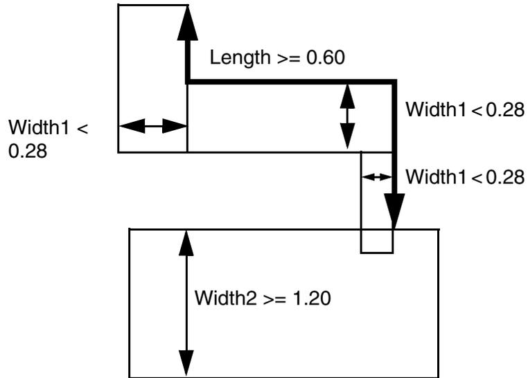
a) Okay; length  $\geq 0.60$  among all protrusion wires.
