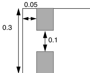
f) Okay. Extra cut is  $\leq 0.2$  away; therefore use min-width rule, and both cuts meet the min-width enclosure rule of 0.0 0.05.
