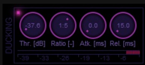
Figure 20: A small sidechain compressor included in Reflectosaurus.
