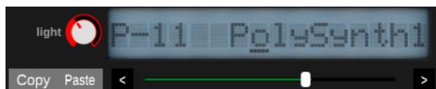
You can modify the tone name by using < and > to navigate through the name. The green slider can be used to change the underscored character.
